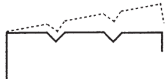
Distortional buckling of the edge stiffened element
