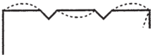
Local sub-element buckling
