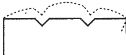
Distortional buckling of the intermediate stiffeners
