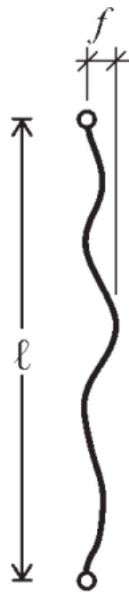
variation of deviation from straightness
